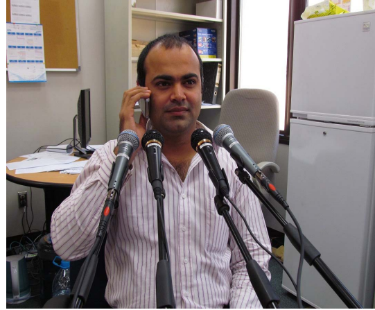
Figure 1. Microphones and mobile phone setup in office environment.
